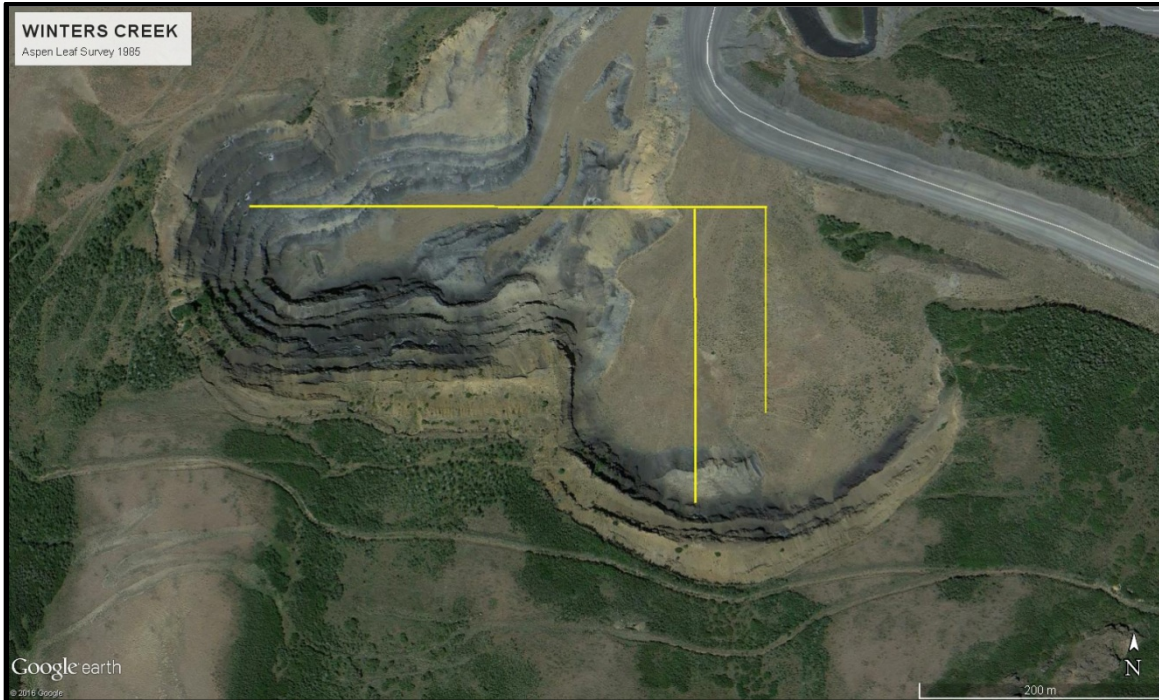
Fig 4. Biogeochemical and mercury soil gas (GASic) survey lines (1985) at Winters Creek, superimposed onto the current mine workings. Survey line locations are approximate.
